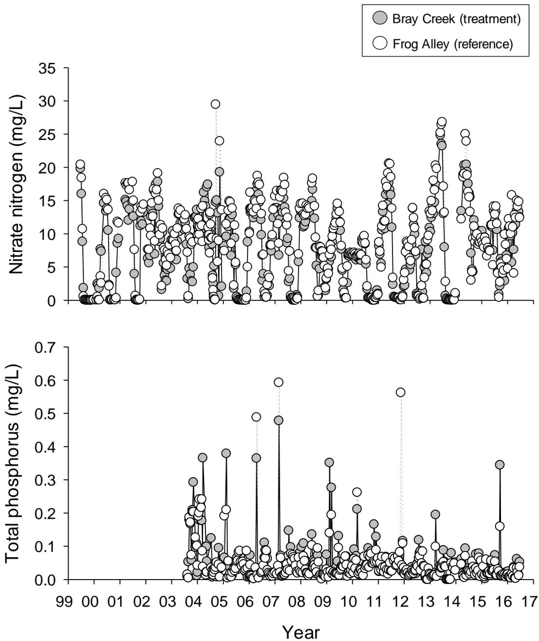
**Figure 6.** Nutrient concentrations for nitrate-nitrogen (NO<sub>3</sub>-N) (top) and total phosphorus (TP) (bottom) from downstream monitoring sites in Bray Creek (treatment) and Frog Alley (reference) watersheds. Concentrations are based on biweekly samples collected between June 1999 and June 2016.
