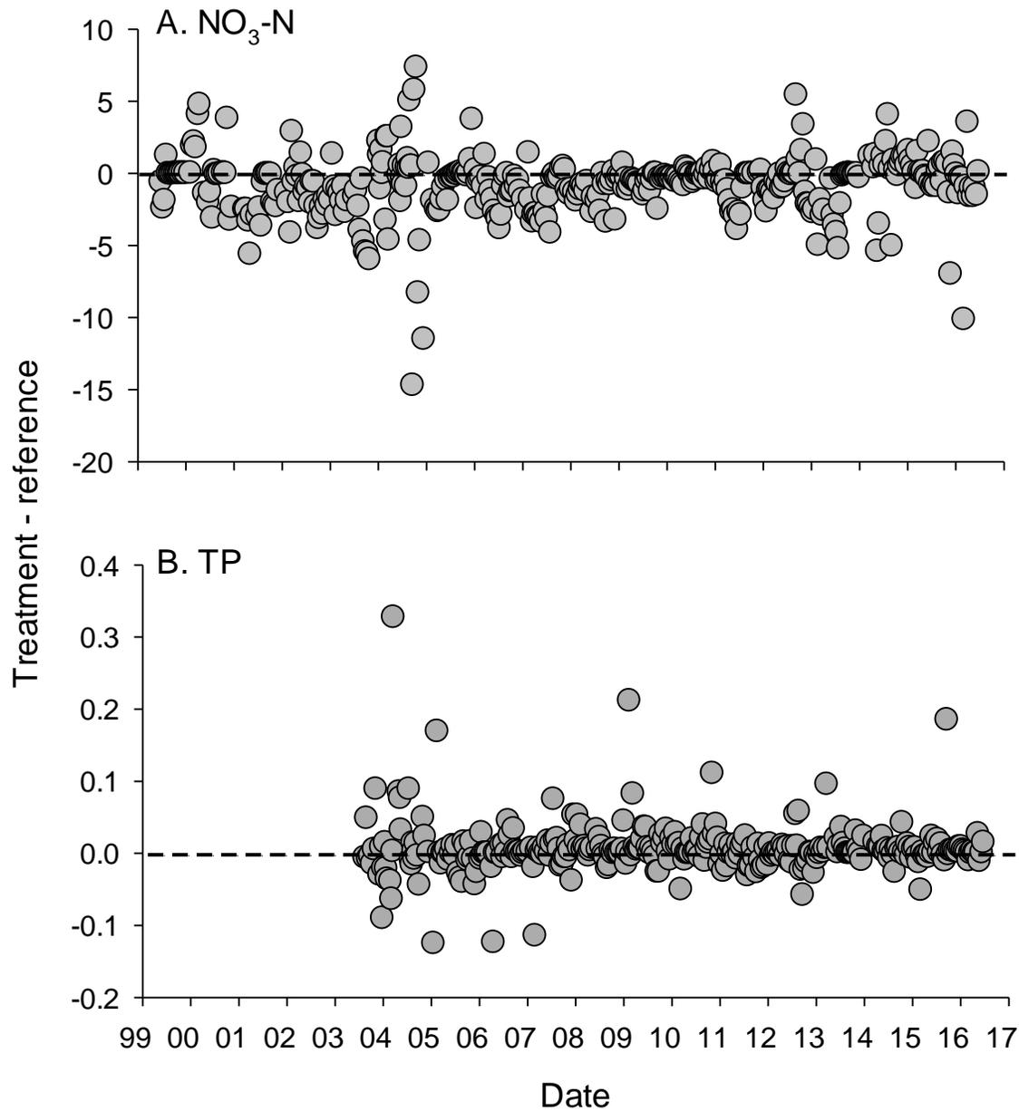
**Figure 8.** Differences between concentrations of nitrate-nitrogen (NO<sub>3</sub>-N) (A), and total phosphorus (TP) (B) in water samples collected at downstream monitoring sites in Bray Creek (treatment) and Frog Alley (reference) watersheds.
