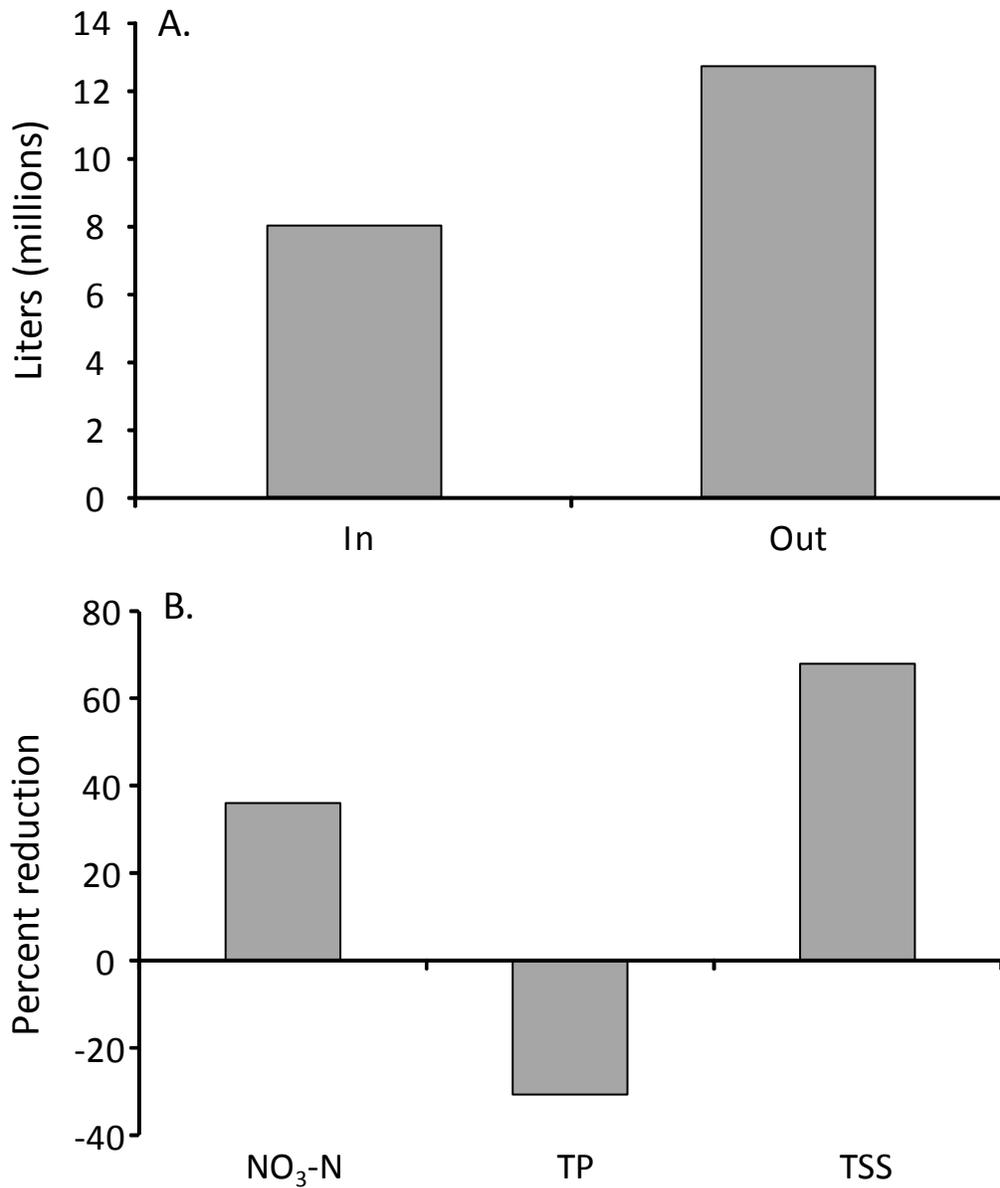
**Figure 3.** Total water inputs and outputs into Arrowsmith North wetland (A), and percent reductions in nitrate-nitrogen (NO<sub>3</sub>-N), total phosphorus (TP), and total suspended solids (TSS) loadings (kg) (B) between November 17, 2015 and May 16, 2016.
