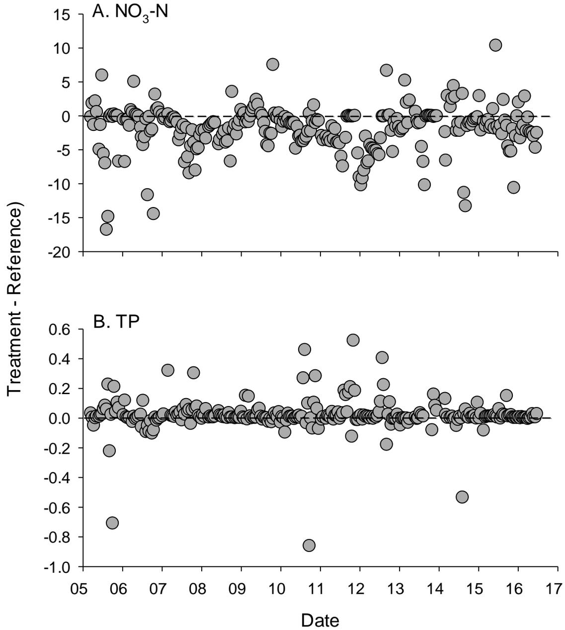
**Figure 9.** Differences between concentrations of nitrate-nitrogen (NO<sub>3</sub>-N) (A), and total phosphorus (TP) (B) in water samples collected at upstream monitoring sites in Bray Creek (treatment) and Frog Alley (reference) watersheds.
