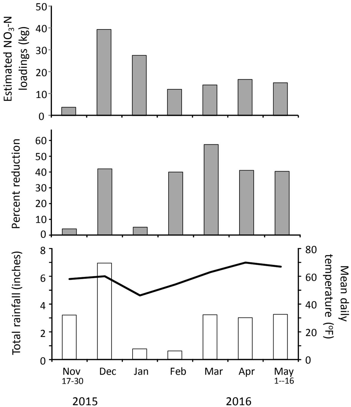
**Figure 4.** Estimated nitrate-nitrogen (NO<sub>3</sub>-N) loadings (top), percent reduction of NO<sub>3</sub>-N (middle), total rainfall (columns) and mean daily temperatures (line) (bottom) by month for the Arrowsmith North wetland constructed in Bray Creek watershed (treatment).
