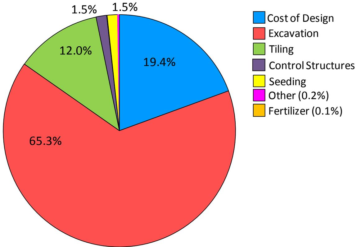
**Figure 10.** Breakdown of total installation costs for CP39 wetlands constructed in two subwatersheds of the Mackinaw River, Illinois. Total costs include actual expenditures from 7 wetlands constructed between 2012 and 2015, and estimated expenditures for 3 new wetlands that will be constructed in 2016. This figure was developed by The Nature Conservancy’s NatureVest team.
