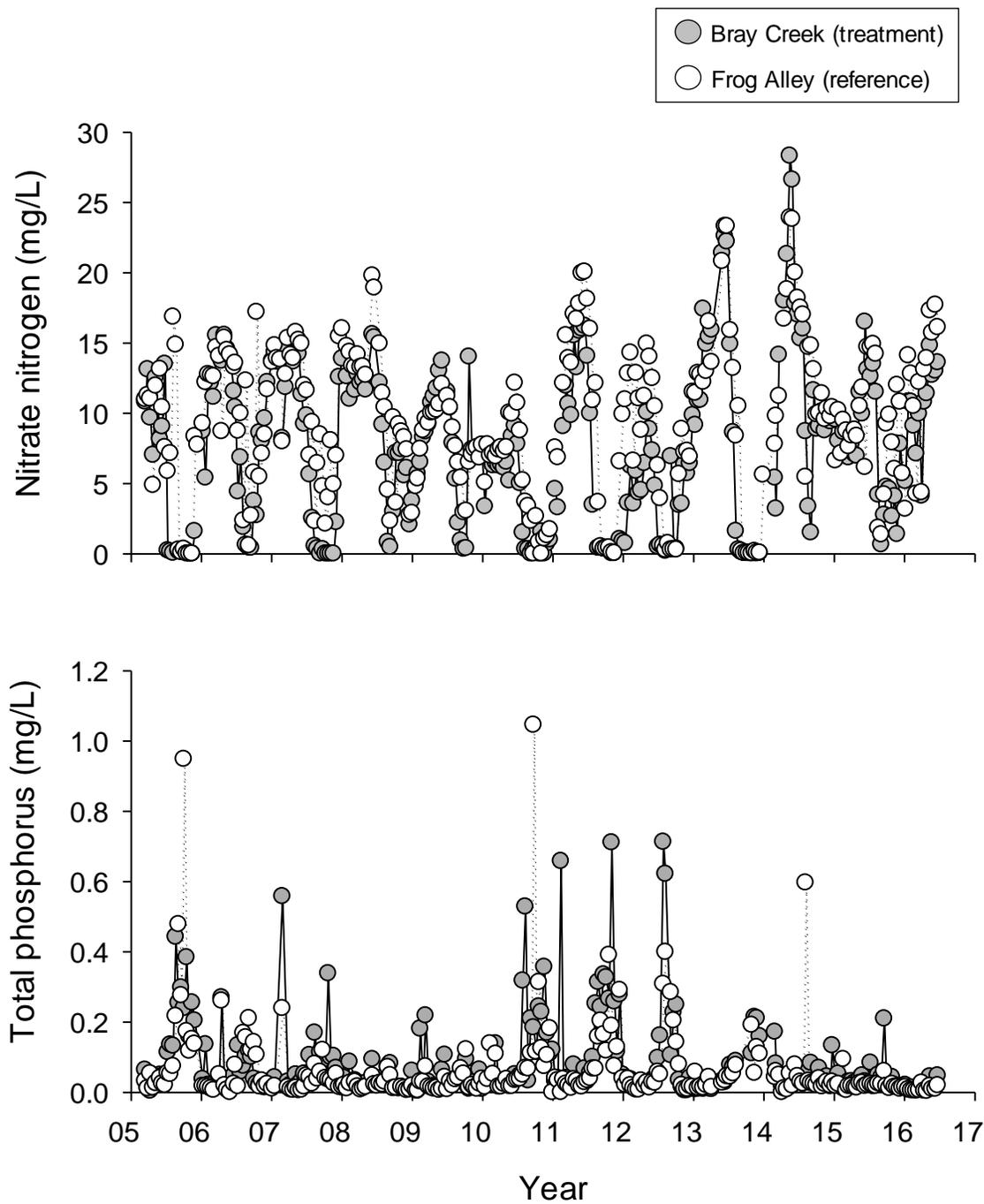
**Figure 7.** Nutrient concentrations for nitrate-nitrogen (NO<sub>3</sub>-N) (top) and total phosphorus (TP) (bottom) from upstream monitoring sites in Bray Creek (treatment) and Frog Alley (reference) watersheds. Concentrations are based on biweekly samples collected between June 1999 and June 2016.
