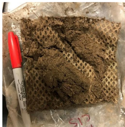
Figure 2.4. Mesh erosion pad installed in a cropped field (left image). A mesh pad with a dried soil sample before being sieved to collect the weight (right image).
