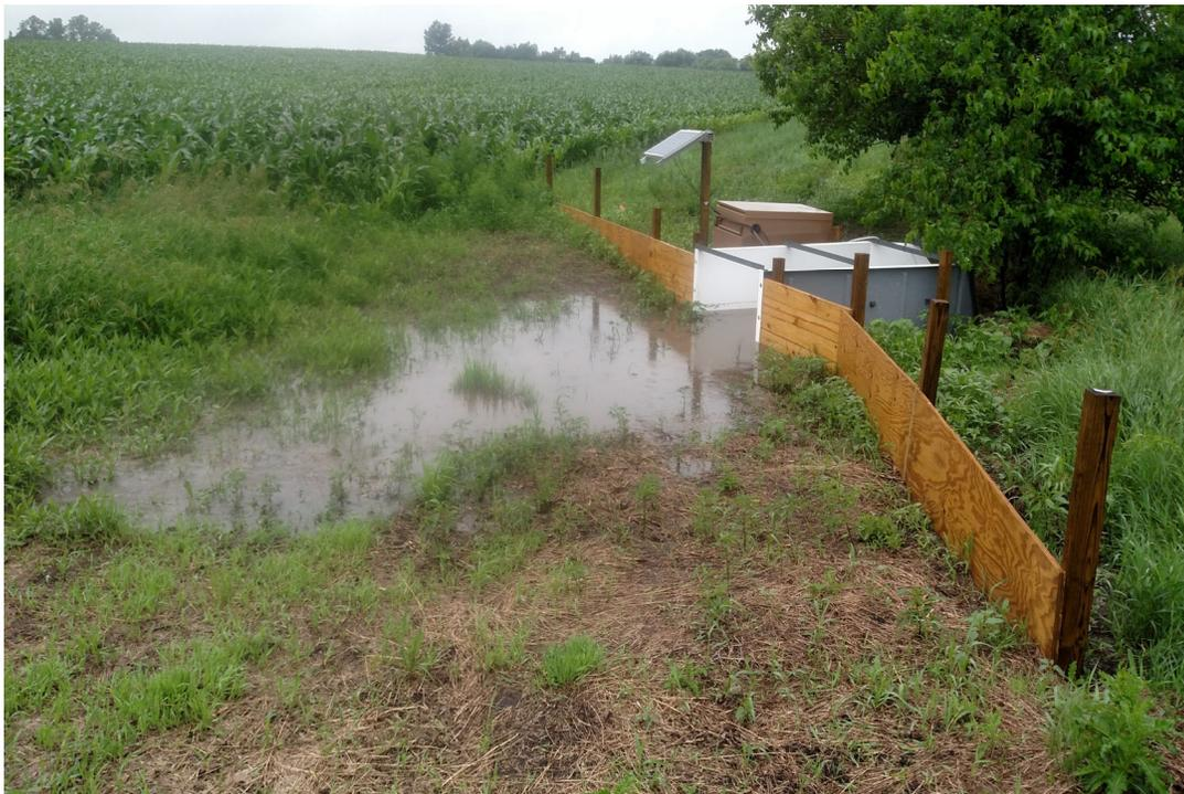
**Figure 2.7.** Surface runoff monitoring collection design with H-flume with autosampler protected inside job box.
