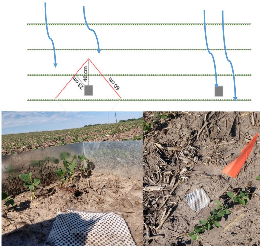
*Figure 2.5. Illustration of paired pad study where one pad had a v-diverter installed upslope from it (left image) paired to a pad location with no v-diverter upslope (right image) in order to gain insight into the type and amount of erosion contributed by local splash erosion processes as opposed to transport through erosion types like sheet and rill erosion.*
